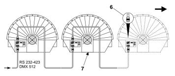
The connection between projector and control unit and between several projectors must be made with a shielded two-pole cable with Cannon 5 PIN XLR plug and socket at the ends.
