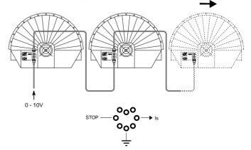
The connection between projector and control unit and between several projectors must be made with a shielded two-pole cable with Cannon 5 PIN XLR plug and socket at the ends.
