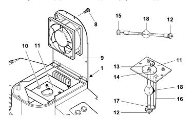
**IMPORTANT:** to ensure maximum uniformity of the light beams, the light bulb must be located with protuberance (**18**), visible on the bulb, pointing towards the rear of the projector.
