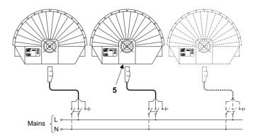
The projector is set up to operate at the power supply voltage and frequency shown on the electrical data label (5) on the back of the projector itself. Ensure that these values correspond to the electricity mains network voltage and frequency.
