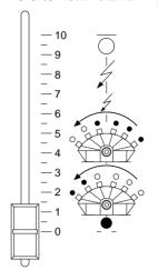
With the cursor at 0% all bands are obscured. In the cursor interval between 0% and 25% the bands are progressively opened from right to left, creating a fan effect. From 25% to 54.7% the bands are progressively obscured from right to left. From 54.7% to 95% a strobe effect is obtained with an increasing frequency from 1 flash every four seconds to 2 flashes/second. The aperture is fixed from 95% to 100%.
