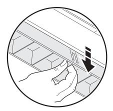
4. The diffuser is held in place by metal clips at each end of the luminaire. Push a clip back and remove the diffuser. You now have access to the tubes.
