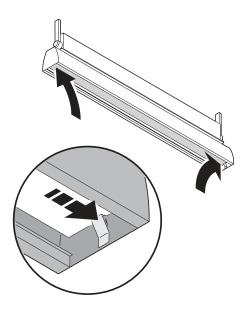
Pressing on the metal caps at both ends of the tube, rotate the tube 1/4 turn in whichever direction is easiest, and slide the tube's terminal pins out of their sockets. Support the tube at both ends as it is released.
