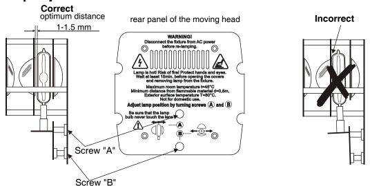
The lampholder is aligned at the factory. Due to differences between lamps, fine adjustment may improve light performance.
