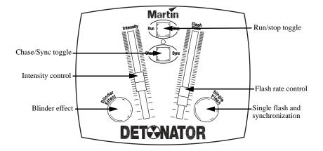
The optional Detonator remote control provides the following:
